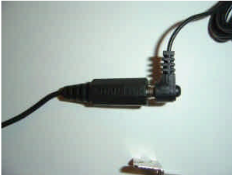
Figure 1-D AC/DC Power adapter plugged into All-In-One Cable
