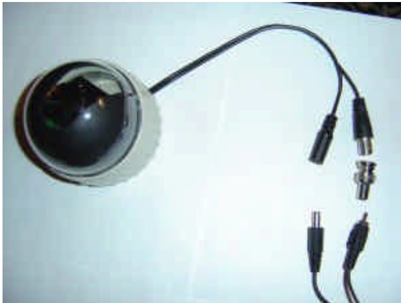
Figure 2-E CCD Camera shown laid out before connecting Cable Note: Cables would normally be routed inside the wall with a Dome camera, shown for instructional purposes only.
