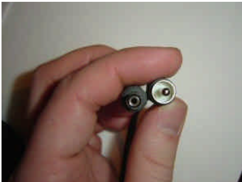
Figure 2-A Camera end of All-In-One Cable with 1 power lead (Left) and 1 RCA Video Connector (Right)
